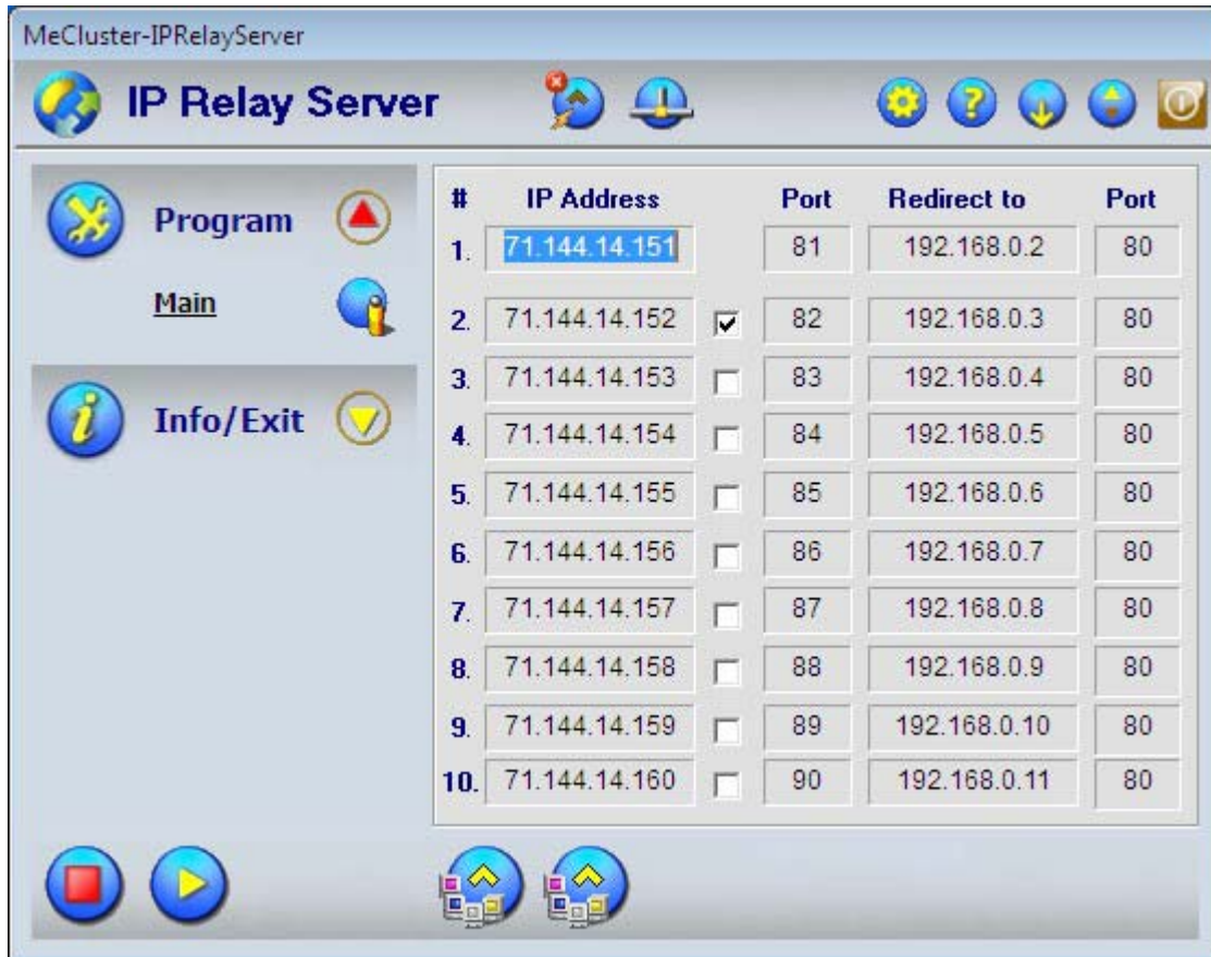
Figure 2.2.4 IP Relay Server Development Environments
